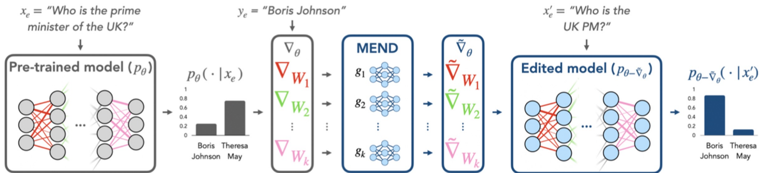
Figure 1: The proposed algorithm MEND enables editability by training a collection of MLPs to modify model gradients to produce local model edits that do not damage model performance on unrelated inputs. MEND is efficient to train and apply edits, even for very large models, as shown in Section 5.1.
